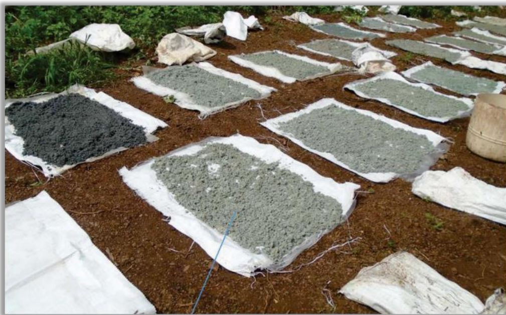
Figure 10.8.10 Drying Wet RC Samples (Newcore, 2017)
