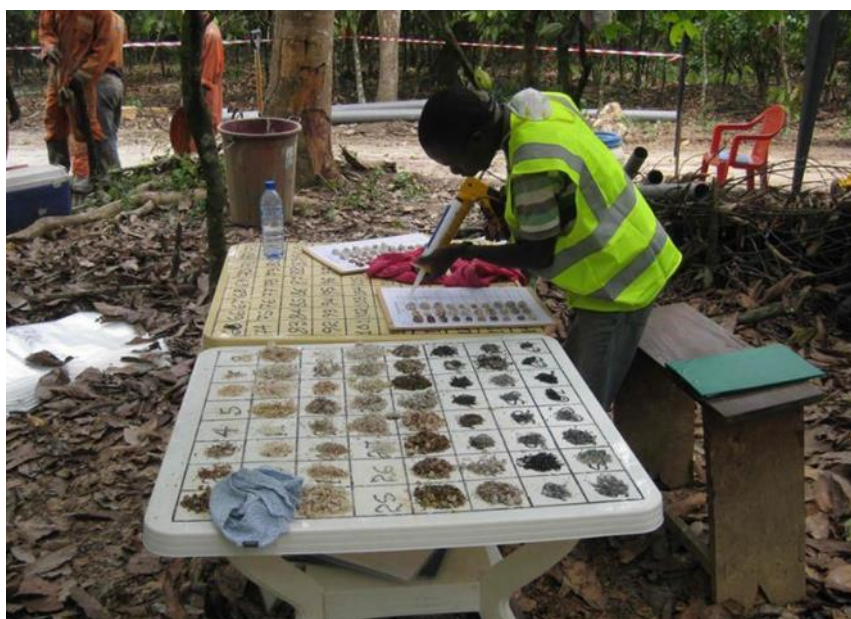
Figure 10.8.6 Chip Board Preparation (Newcore, 2017)
