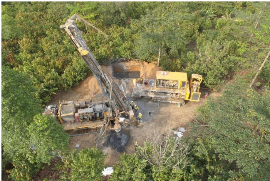
Figure 10.8.3 Reverse Circulation Drill (Newcore, 2021)
