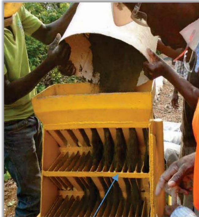
Figure 10.8.9 Reverse Circulation Sampling Riffle Splitter (Newcore, 2017)
