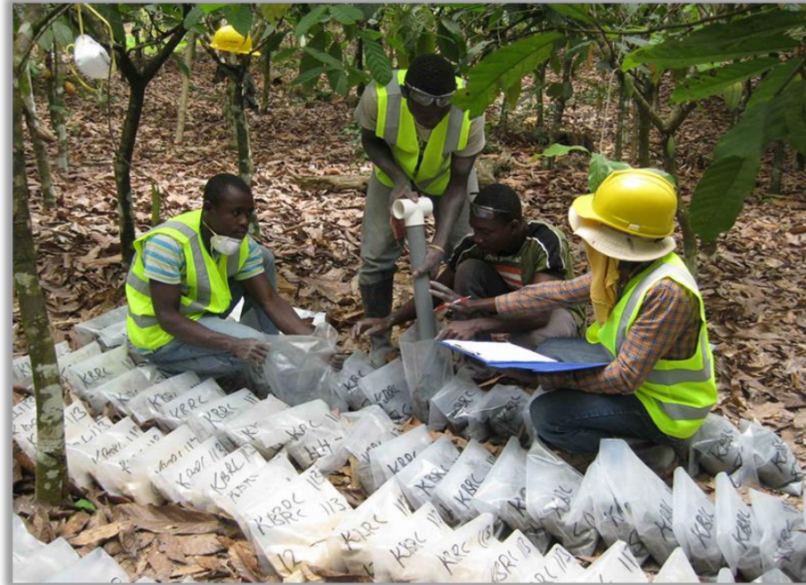
Figure 10.8.9 Reverse Circulation Sampling Riffle Splitter (Newcore, 2017)
