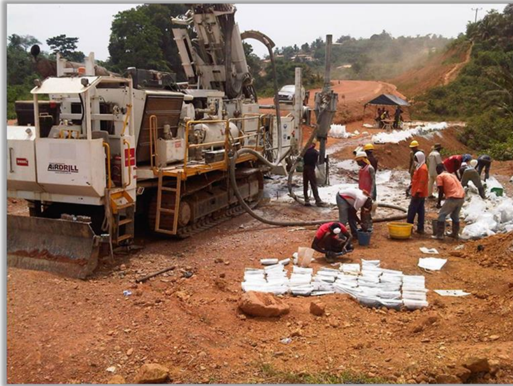
Figure 10.3.1 Reverse Circulation Drill (Newcore, 2012)
