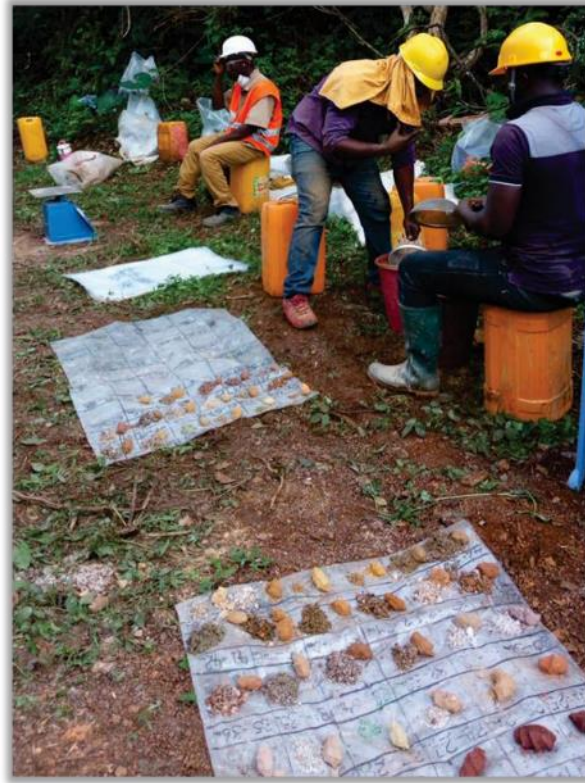
Figure 10.8.6 Chip Board Preparation (Newcore, 2017)
